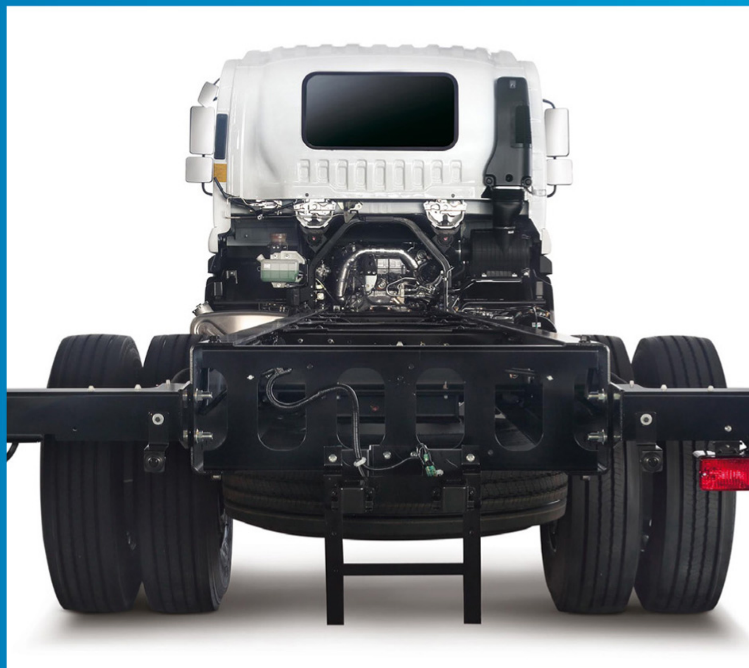
Rivetless wider chassis for greater ease of body-building installations.
