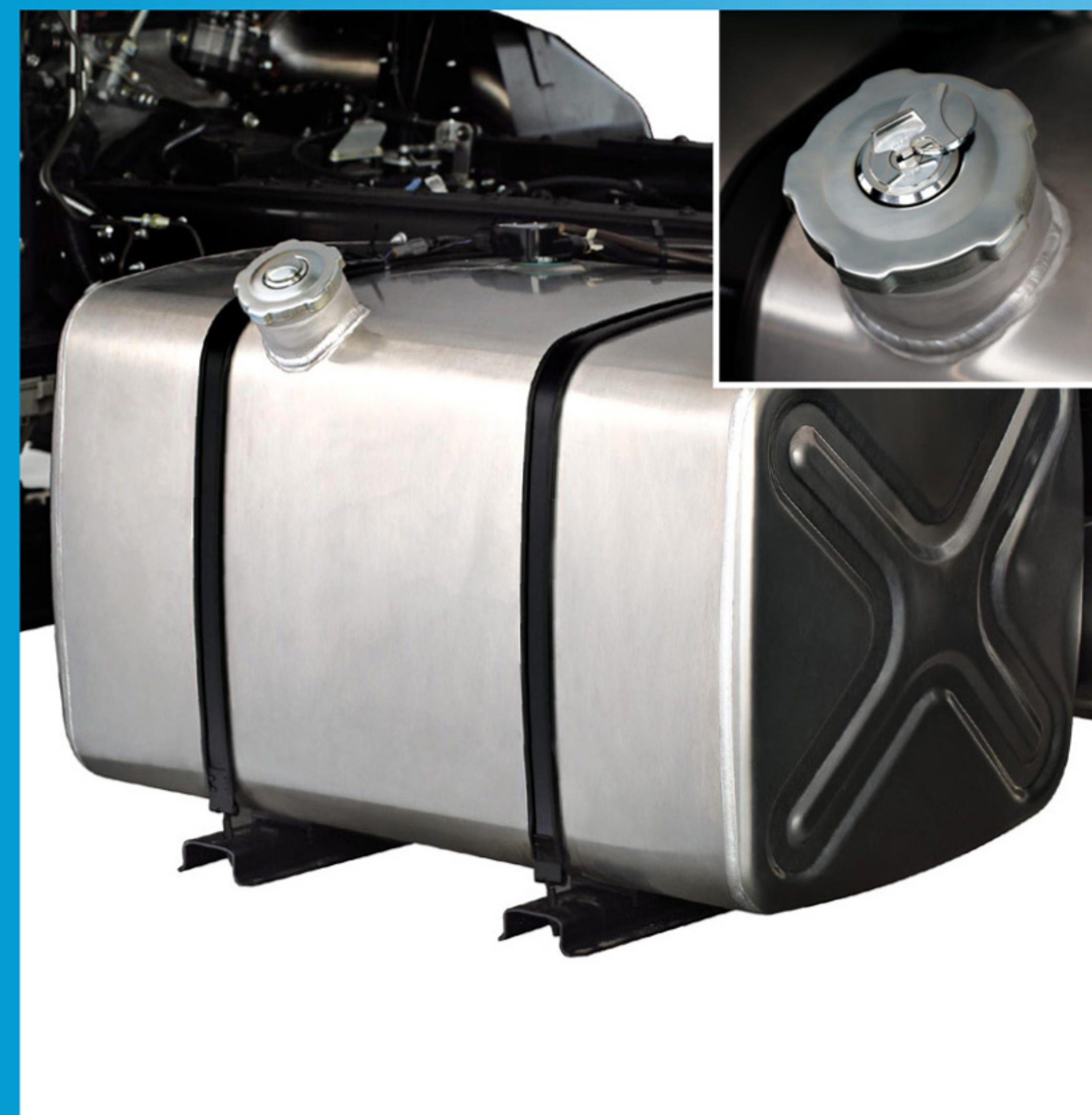
Bigger and durable aluminium alloy fuel tank with lockable cap (Applicable to FVR34UU-SD & FVR34UU-ST2).
