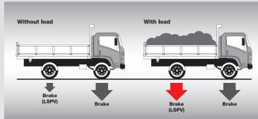
▲ Load sensing proportioning valve (LSPV).
