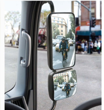
Wide-angle mirror offers extra visibility of surroundings and minimising blind-spots.
