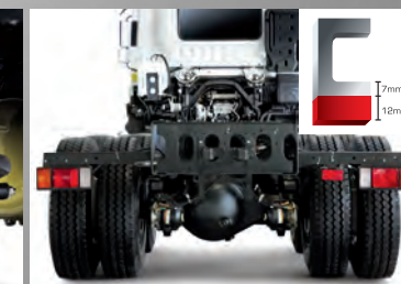
▲ Bigger axle capacity with reinforced frame chassis (12mm).
