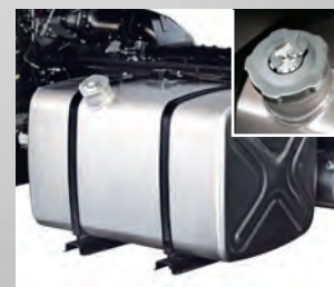
▲ Bigger and durable aluminium alloy fuel tank with lockable cap.
