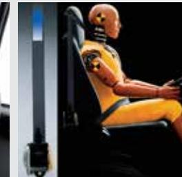
\*SRS airbag system and seat belt with pretensioner are activated in the event of a frontal collision, mitigating impact to the head and chest.
